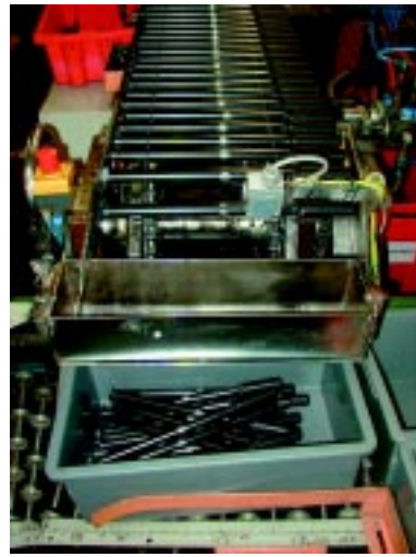
... into pump shafts which then drop into a box ready to go for packing
