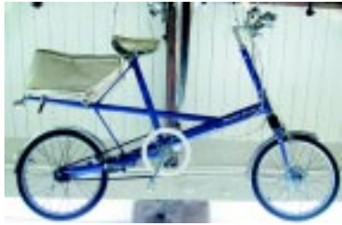
left: It has dual suspension, big luggage carrying capacity and rides like any other quality bicycle - The Moulton. above right: early-day ways of carrying your Primus pressure stove. right: a steel advertisement panel for the 1902 patented hub gears that help you travel easy.
